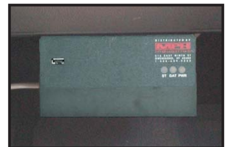
Recorder installed below glove box
